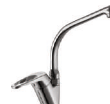
RR-3301 MRP 7435/- Single Lever Sink Mixer with High Swivel Spout (Side Operated) with 450mm Long Flexible Connectors, Deck Mounted
